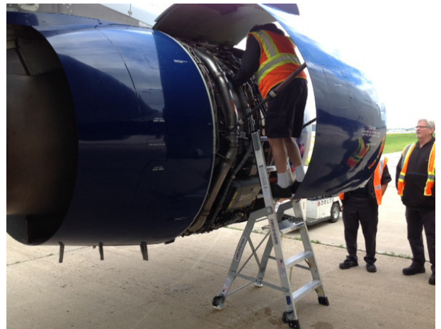
The 6LNCPYLON allows close working access under the engine cowlings, aircraft pylon areas and in the engine shop.
