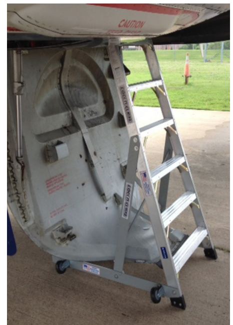
8WWCADET allows stable working access to gear and wheel well electronics and maintenance points.
