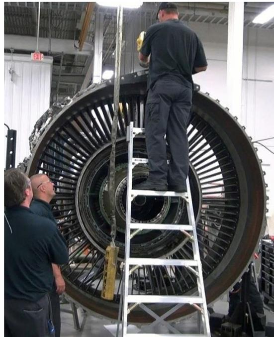
**MRO technicians (left) use an A-frame ladder which requires twisting the torso which puts torquing pressure on the spine. LockNClimb's PYLON ladder (right) allows the technician to face his work directly and maintain an ergonomically correct position.**
