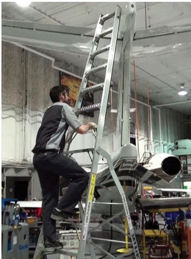
***MRO technician at Duncan Aviation in Lincoln, Nebraska, uses a sturdy free-standing LockNClimb 13LNCPYLON to service the tail elevators on a corporate jet.***
