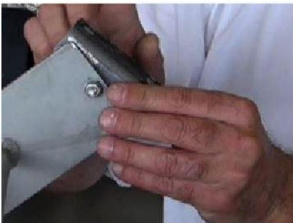
***This ladder has a missing rubber foot and is Potentially dangerous.***
