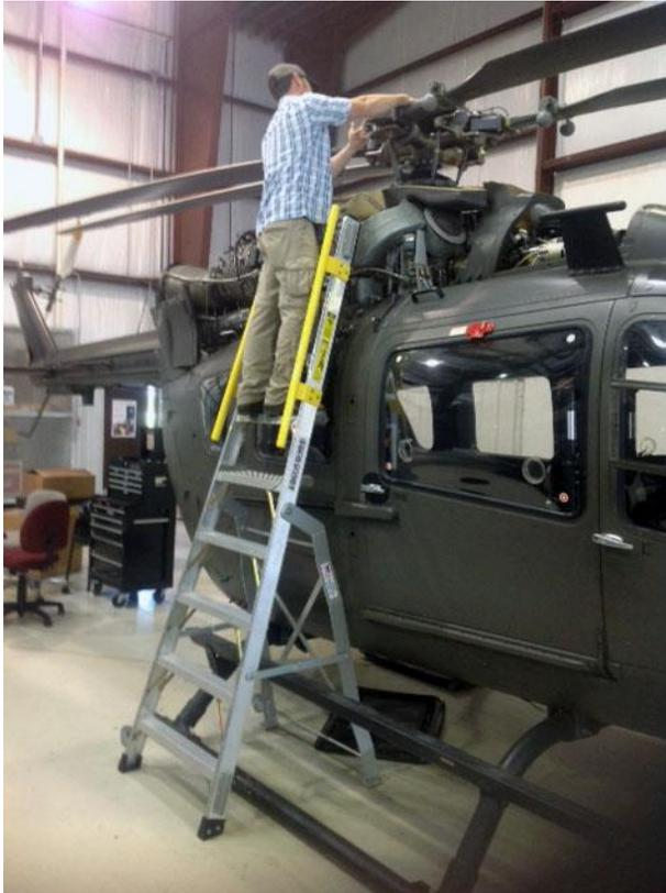
***MRO technician uses LockNClimb's 9HELIPYLON to Service top engine rotor on a UH-72 Lakota used by the U. S. Army. Notice how the wide treads provide comfort while standing, how the ladder has been specifically designed to fit over the skids, allowing the technician to ergonomically face his work "between the rails."***
