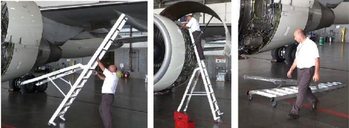
***Walk the ladder up to the desired position. Work within the rails to help avoid back and spine injuries. Always lay the ladder flat on the surface when leaving the work area.***
