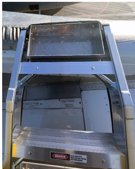
Built in TOOL TRAY at the top of the ladder facilitates quick repairs and maintenance tasks as tools and parts are staged next to the work area.
