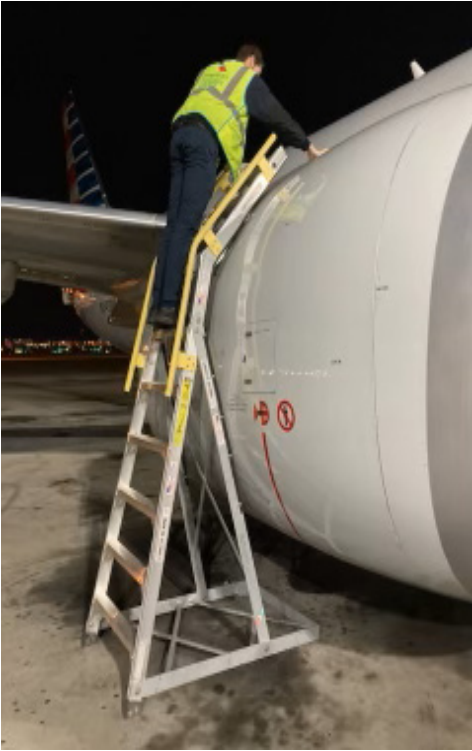
10COWLPYLON737MAX rolls easily on hard rubber wheels and slides in place on brass feet to allow safer working access to the service panels on top of the engine pylon area of B737NG and B737MAX.
