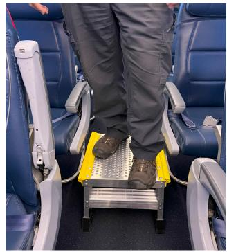
Mechanics no longer have to stand on seats or armrests to reach overhead bins or service lights and electronics.
