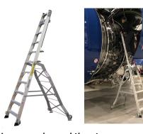
Lower engine and thrust reverser, higher nose gear area.
