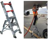
GPU port, all purpose ladder for reaching lower exterior.
