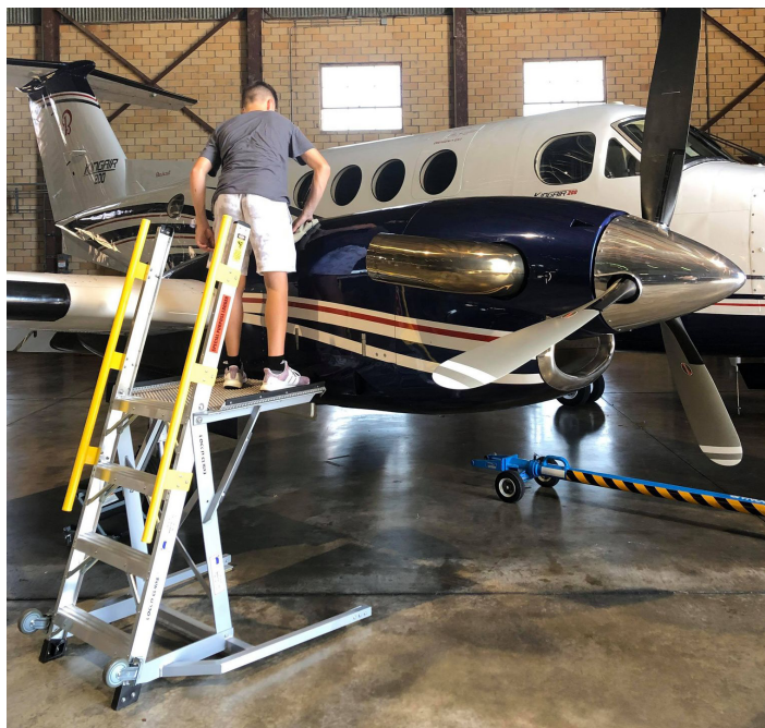
44LNCPLAT provides a wide stable platform for many service and cleaning applications around fuselage.
