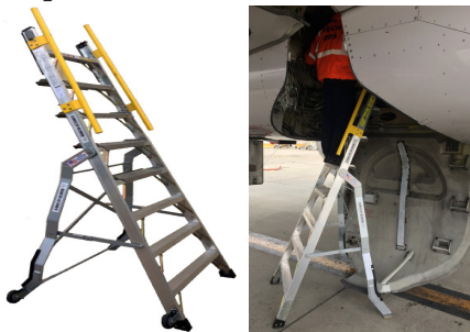
Step through access into cargo hold baggage bays.
