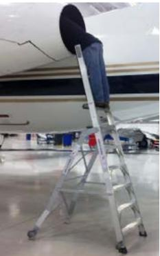
**11LNCPYLON** allows technicians to perform MRO service from a stable, ergonomic position. Maintenance and repairs on the engines can be accomplished by working "within the rails" without twisting the spine which can lead to many back-related injuries. This free-standing ladder achieves top support by protective padding.
