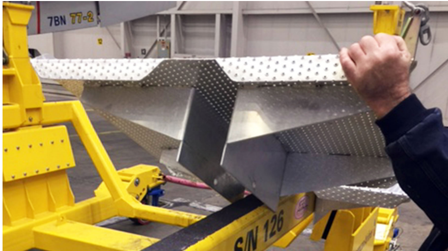
The LOCKN-WALK fits securely over the horizontal rail of the engine stand.
