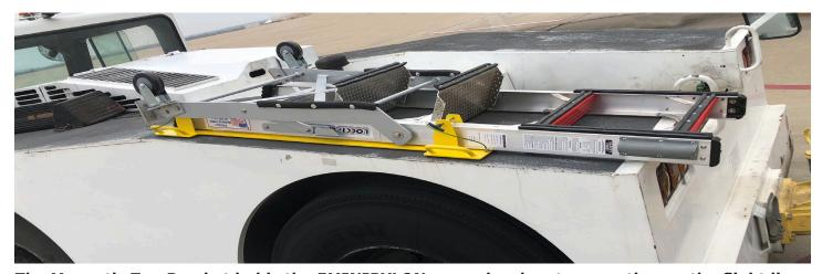
The Magnetic Tug Bracket holds the 5MINIPYLON securely when transporting on the flight line.
