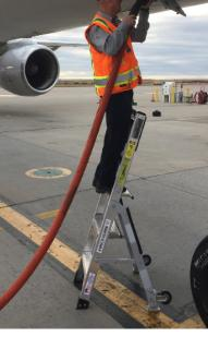
The 5MINIPYLON is used to service the GPU ports, lower thrust reversers, lower fan cowl area, wheel well area, or nose gear of the Boeing 757 & 767, MD 10/11 and the Airbus A300 series.
