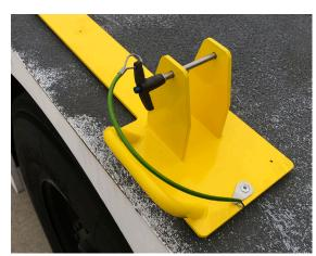
Push pins secure the 5MINIPYLON inside the brackets.
